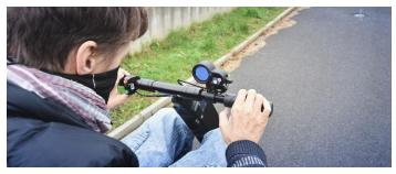
Control the accelerator by tilting the handlebars towards, brake by moving away from yourself.
